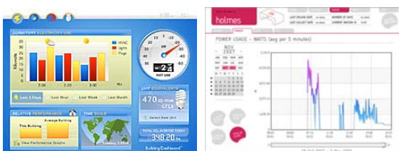
Figure 4. Lucid Building Dashboard (left) [5] and Holmes [7] (right) allow dwellers to explore in detail the patterns of consumption within their home or building.
